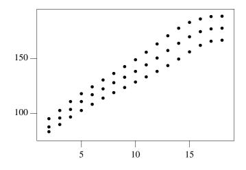
Because there are four numbers on each input line, the first is taken as an *x*-value and the remaining three are plotted as *y*-values.
