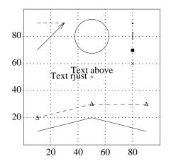
This figure also illustrates the combined use of the draw and next commands. Saying draw A solid defines the style for a connected sequence of line fragments to be called A. Subsequent commands of next A at *point* add *point* to the end of A. There are two such sequences active in the above example (A and B); note that their next commands are intermixed. Because the predefined string delta follows the specification of B, that string is plotted at each point in the sequence.
