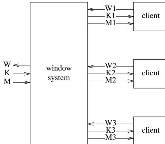
If the window system multiplexes clients of its own type, then it may be a client of itself, or a client may pass its environment to a fresh invocation of the window system to do further multiplexing. This recursion allows a client of window system — a text editor, say — to invoke the window system afresh in its window to manage subwindows for multiple views of files being edited.
