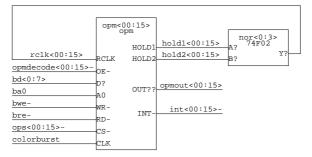
Sixteen copies of the opm circuit are made. The pattern D? is at a lower, i.e., "faster running," level than opm<00:15>, with the effect that all the D0's are connected to bd0, all the D1's are connected to bd1, etc; similarly, all the A0's are connected to ba0. On the other hand, all the CS-'s are separate: opm00/CS- (the instance of CS- in opm00) is connected to ops00-, opm01/CS- is connected to ops01-, etc. The manual entry for *cdmglob* should be consulted for all the details.
