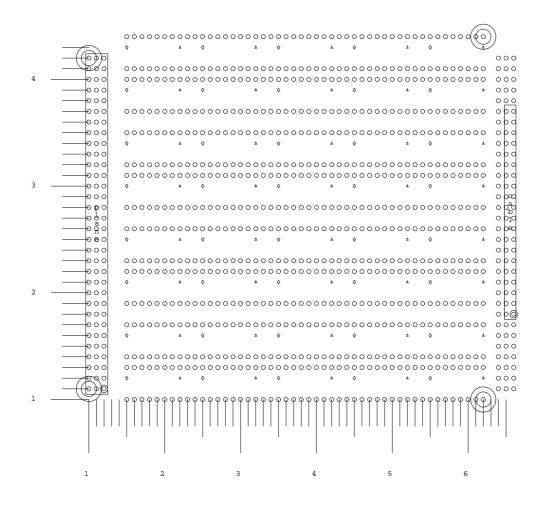
Note how the alignment marks are shown. Pin 1 of each package is illustrated by two concentric circles around the pins. Now a wrap file (with extension .wr) suitable for driving the semi-automatic wire-wrap machine can be created with *wrap* -*cv*. The use of Multiwire technology needs some hand holding – consult an expert.
